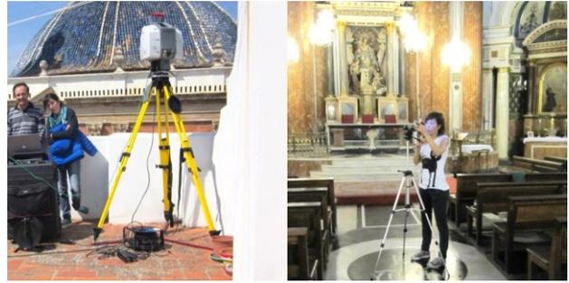
Figure 3. The survey with laser scanner and thermal camera
