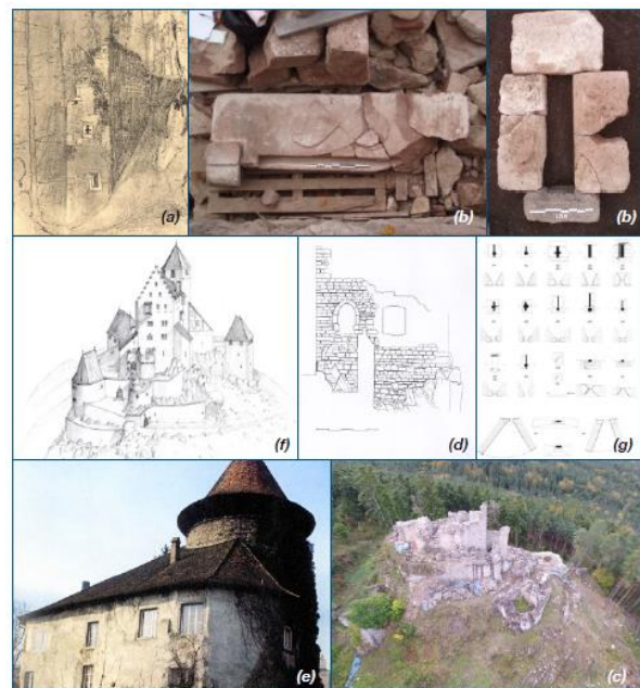
Figure 3: Collected data as a support the modeling (a) iconographic documents; (b) and (c) photographs; (d) digitalization on orthophotos; (e) photographs of similar sites or roof structures; (f) and graphical restitution propositions
