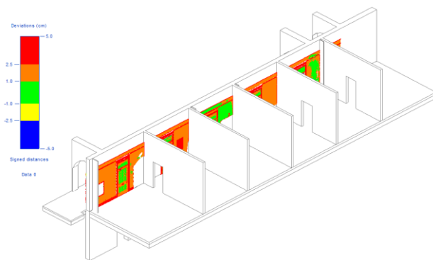
(a) Analysis of deviations before wall replacement
