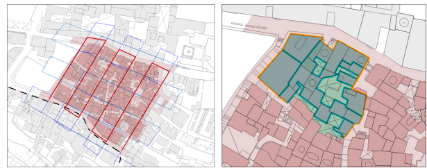
Figure 6: On the left, flight plan set with DJI Phantom 4 Pro for each area, where the 5 missions are marked (one with a 90 ° gimbal angle, the other 4 with 45 ° angle directions). The flights has been set at 34 m high from the ground level. On the right, close range photogrammetry of urban fronts (in orange) with SLR camera and integration with data from DJI Spark for the acquisition of detail of courtyard fronts.
