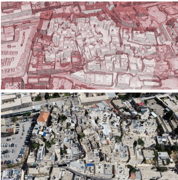
Figure 8: The Agisoft Photoscan visualization of Al-Anatreh 3D model in wireframe and texture mode obtained by DJI Phantom 4 Pro flight plan.
