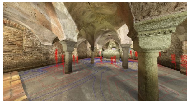
Figure 5. Example of a dimensional analysis of the flooring performed with EasyCUBE PRO: Advanced 3D model of an historical building
