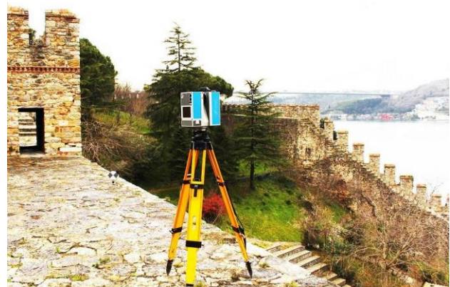
Figure 2. The terrestrial laser scanning system Z+F IMAGER 5010 at the fortress Rumeli Hisari (Courtesy of Solvotek Mühendislik)
