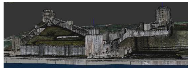
Figure 4. Final result of solid modelling in 3ds Max – the fortress as a polygon model with textures
