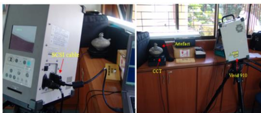
Figure 4. Scanning of artefact using VIVID 910 scanner
