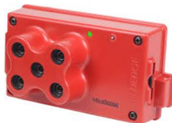
Figure 2: Micasense RedEdge multispectral camera.
