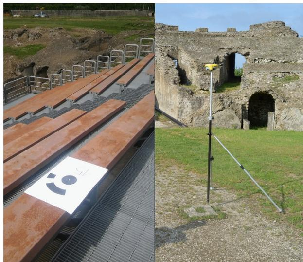
Figure 6: GCP measurement phase: right panel on photogrammetric targets, left panel on natural points.
