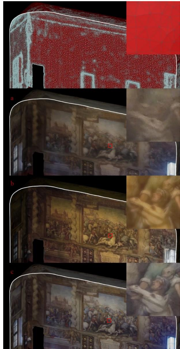
Figure 14. Triangulated surface generated by ZEB point clouds with associated photogrammetric texture. *top*, ZEB triangulated mesh in wireframe view. Texture from: *a*, ZEBcam frames; *b*, Sony ILCE images; *c*, steadicamera frames. For each textured mesh model, a zoomed view of about 50x50cm.
