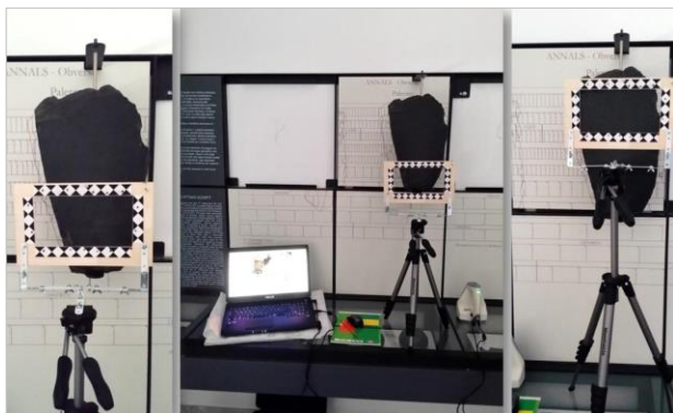
Figure 2: Acquisition phases via 3-D scanning of the Palermo Stone.
