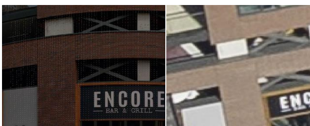
Figure 7. Original image projections of MM [left] and aerial oblique image [right]. Please note the grey dots in the left hand image - these are projected grid cells used for the extraction of image information
