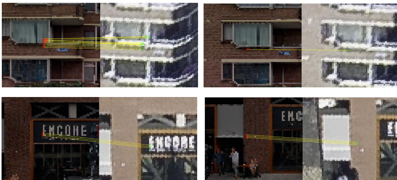
Figure 9. Four exemplary registration results between MM and aerial oblique images. The MM images are on the left hand side, the aerial oblique images on the right hand side
