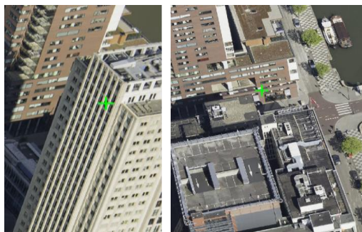
Figure 6. Back-projected patch centre coordinate. Left: False positive of visibility hypothesis. Right: True positive of visibility hypothesis of the same point
