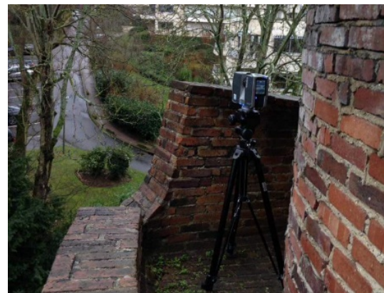
Figure 2 The Faro Focus 3D CAM2 acquiring scans of exteriors
