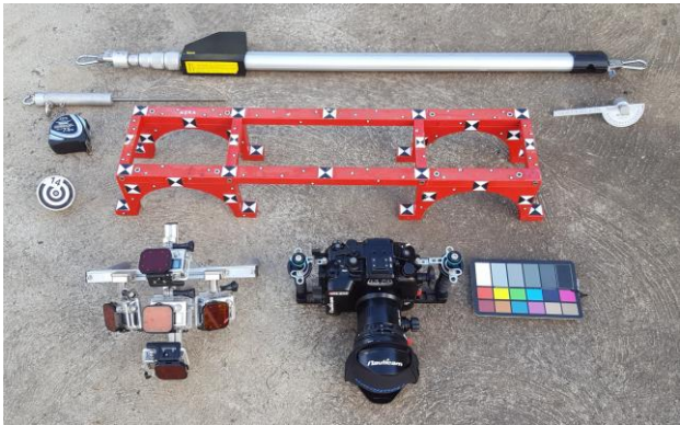
Fig.2: Various devices for underwater measurements of GCPs and for image acquisition. From top to bottom: Graduated telescopic bar for distance measurements; GCP pole with attachment for distance measurements; measurement tape for long distances; calibration frame; device for coarse angular measurements; signalized photogrammetric GCP target, to be fixed to the pole; 5-head GoPro camera system (not used in this paper); Lumix camera with wet lens dome port; chart for color calibration
