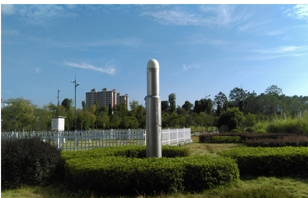
Figure 1. Continuously operating reference station
