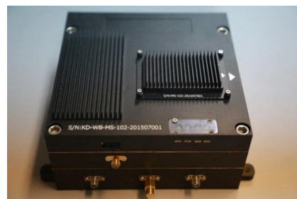
Figure 1. RF and digital subsystems integrated into the enclosure
