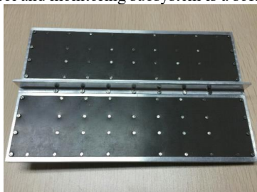
Figure 2. The antenna array of full polarimetric SAR system
