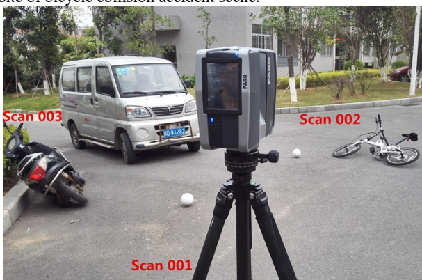
Figure 1. Scanner scans the scene of the accident
