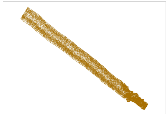
Figure 15. D-P thinning method of 16% thinning rate
