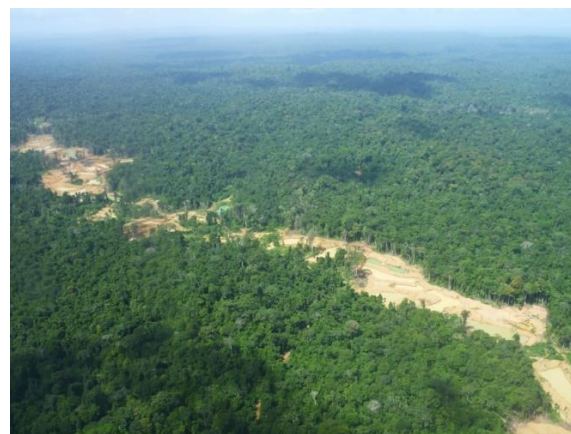
Figure 2. Example of a typical ribbon pattern of alluvial mining practice.
