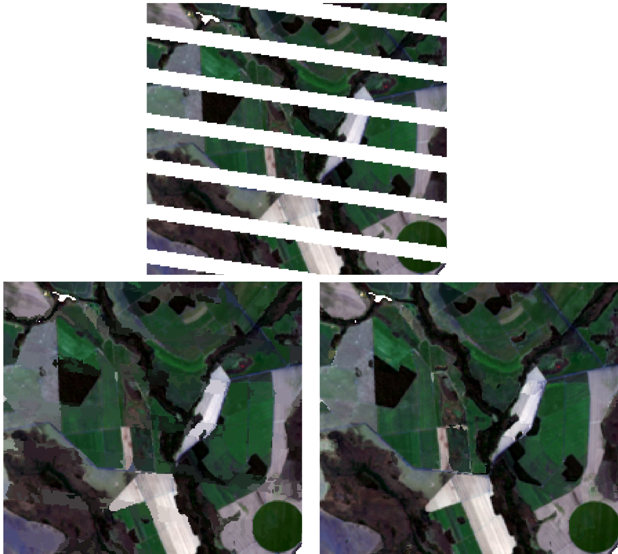
Figure 3: SLC-off Landsat-7/ETM+ image (upper image); image filled through Maxwell et al. (2007) hierarchical multi-scale segmentation method (bottom left image) and the image filled through the proposed method, which uses segmentation pixel weighting (bottom right image).
