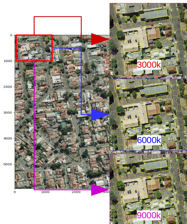
Figure 3. Original image with a detach for a particular region. The impact of different values for k can be verified in the amplified images. Superpixels are in yellow
