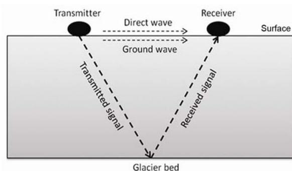
Figure 2. GPR operational principles. Figure is from Singh, 2012.
