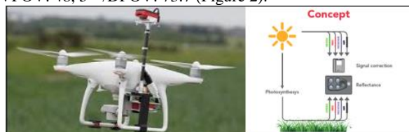
Figure2. Drone Phantom 4 Advanced with integrated Parrot sequoia camera.
