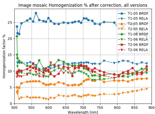
Figure 3. Image mosaic DN homogenization improvement per band of each data set after radiometric correction. FPI band centre wavelengths are marked with circles and triangles.
