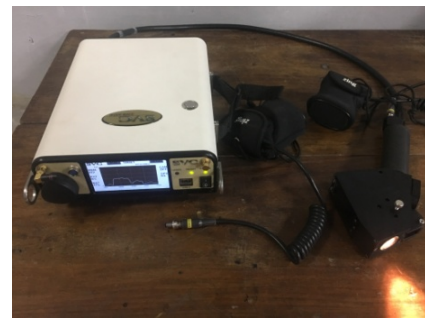
Figure 2. Spectro-radiometer instrument set up
