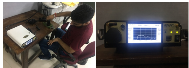
Figure 5. Laser guided spectral reflectance measurement for mango leaves and recorded spectral signature over LCD display
