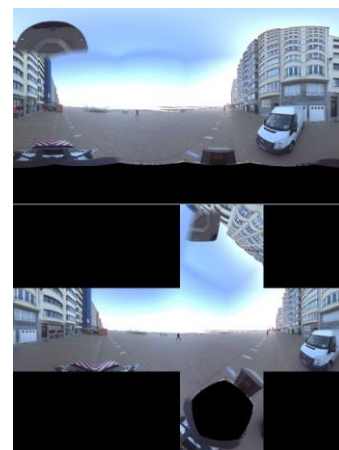
Figure 2. Cube mapping of spherical panorama images allows for more accurate detection of objects For the case of Ostend, on average, 70,000 spherical images were first converted into cube boxes (see Figure 2).
