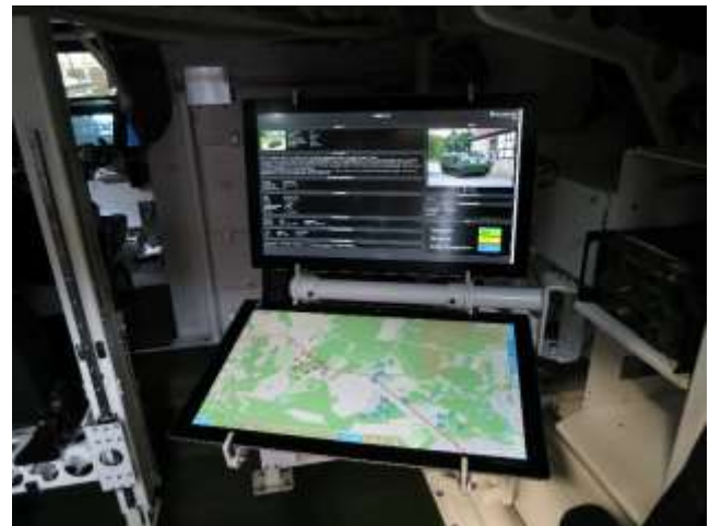
Figure 2: COP example in an APC PMMC G5 from FFG Flensburg, Germany.
