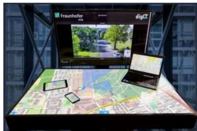
Figure 3: The map is shown on the table display, the additional information is displayed on the vertical display.
