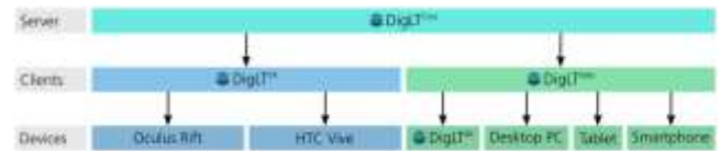
Figure 6: Software components of the DigLT system and possible display devices.
