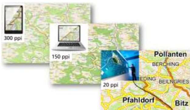
Figure 5: Adaptation of the display to the hardware resolution with the same spatial extent.
