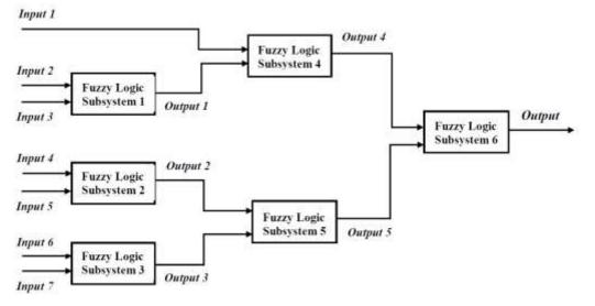
Figure 1. Three-level hierarchical fuzzy logic system
