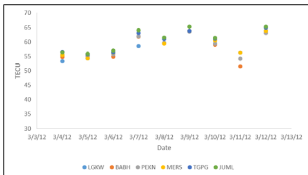
Figure 5. The variation of TEC (in TECU) changes during flare X5.4 for all selected MyRTKnet stations from 3 rd – 12 th March 2012 using GPS_TEC.
