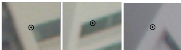
Figure 4. Left is the master image with the keypoint marked. Center and right are slave images with the initial locations of the keypoint
