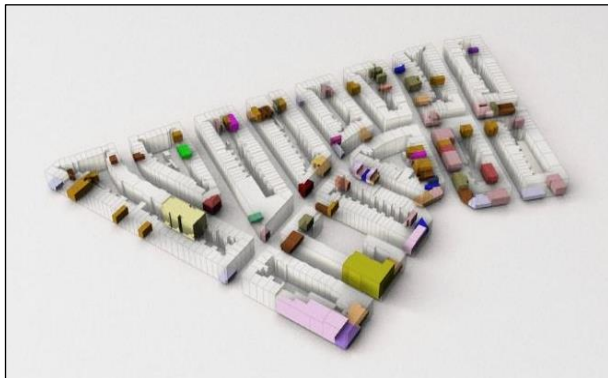
Figure 4. Example of indoor space calculation in Fannius Scholtenbuurt, Amsterdam. Transparent volumes: LoD1 buildings, coloured volumes: non-residential spaces (the colour coding corresponds to the type of space).
