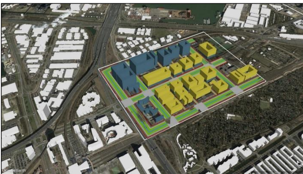
Figure 12. Visualization in CesiumJS of a scenario. Specific attributes can be retrieved by clicking the corresponding building or road element.
