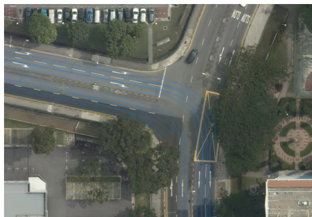
Figure 2. Blue lines indicate the outlines of multiple overlapping scan tracks for a single road.
