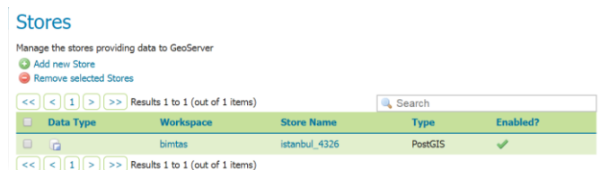
Figure 4. GeoServer publishing spatial data layers from the database through a PostGIS connection.
