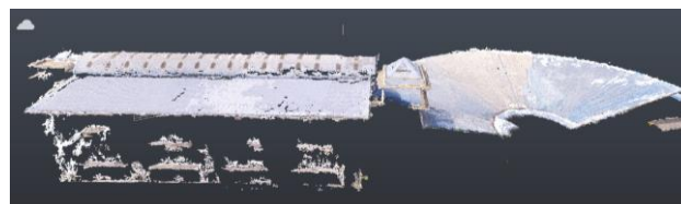
Figure 12 Point cloud of roof generated from Pix4D Software
