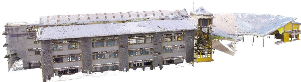
Figure 16 Merged point clouds from UAV and TLS
