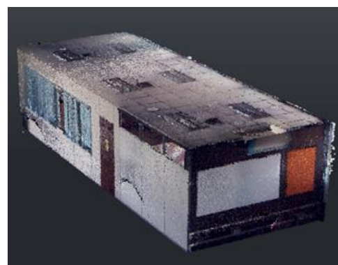
Figure 11 3D point clouds by terrestrial laser scanner
