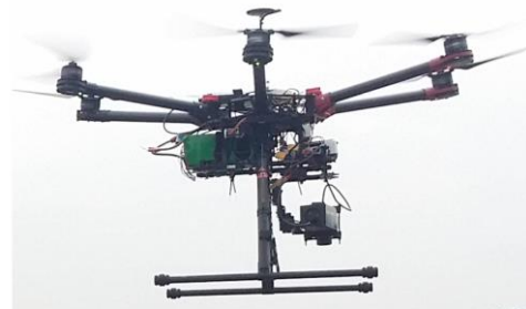
Figure 3: The UAV platform with the hyperspectral sensor on-board.
