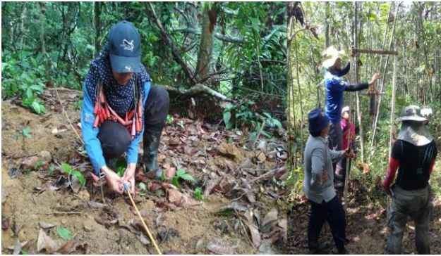
Figure 7 Resistivity and seismic survey
