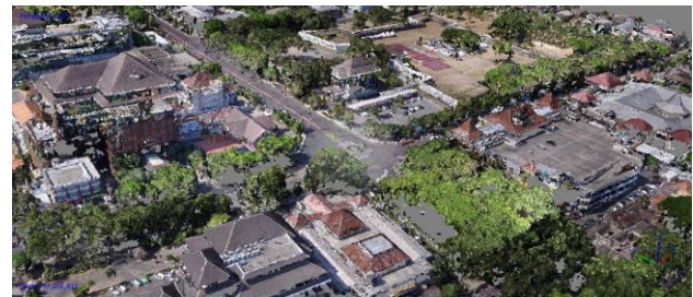
Figure 2. Dense Point Cloud obtained from SfM Processing with Agisoft Metashape
