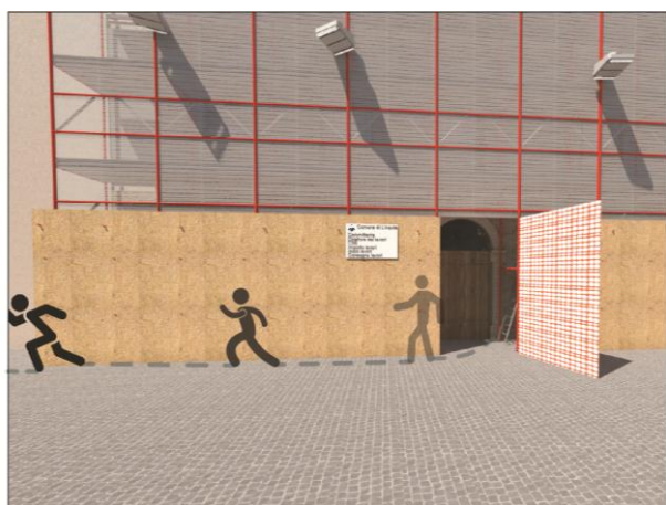
Figure 4. The historic building presents only one way of exodus. In the event that this cannot be used for various reasons such as the breaking of the door or the execution of work activities on the ground floor. The staff will use the stairs provided with the scaffolding to exit and reach the collection point.
