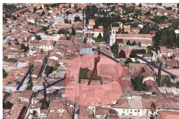
Figure 5. Study of the crane's radius and the presence of other active building site in the immediate vicinity.
