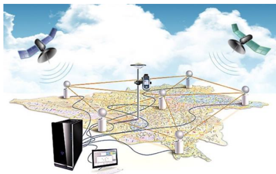
Figure 12: Instantaneous positioning system (Real-time kinematic (RTK) positioning system)
