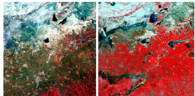
Figure 2: The results of radiometric and atmospheric corrections on Landsat-8 OLI images from 2018 (before flooding, left image) and 2019 (after flooding, right image).
