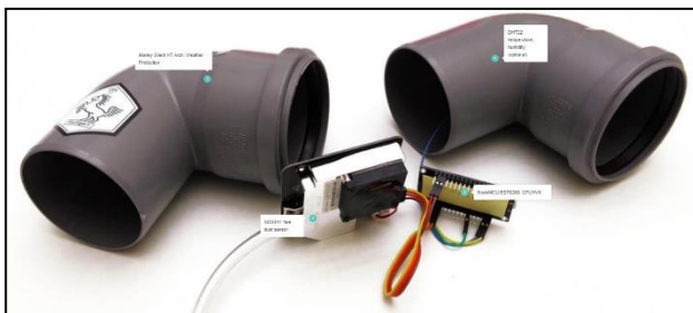
Figure 1. A typical low cost sensor used in the study ( https://luftdaten.info )
