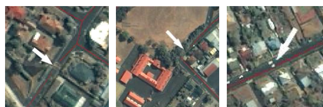
Figure 5. Some small gaps in the extracted road network.
