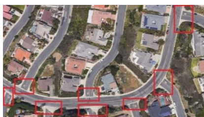
Figure 3. Different colors of road surface in junctions may lead to discontinuities in the extracted roads network.
