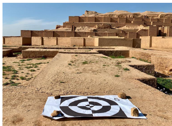
Figure 4. The target used as GCP A5.
