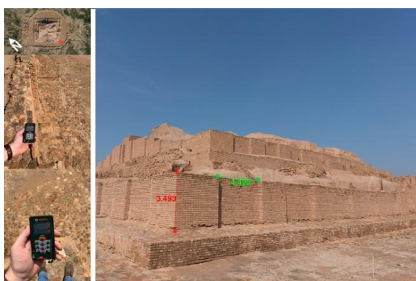
Figure 6. Additional baselines measured on the Ziggurath. On the left side: operation using a hand-held rangefinder; on the right: location of two baselines.
