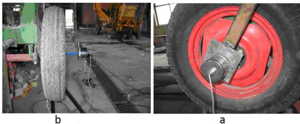
Figure 9. Different views of the encoder mounted on the Seed drill
