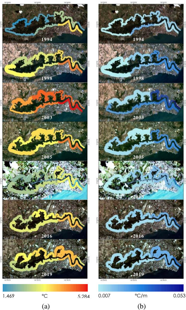
Figure 10. UCI scale and (a) temperature difference and (b) UCI intensity of each zone for each satellite image date
