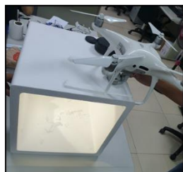
Figure 1. Use of alternative lightbox as an integrating sphere in calibration.
