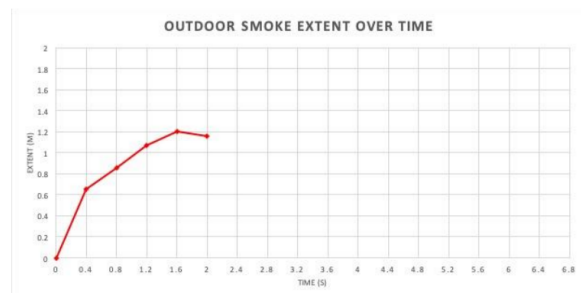
Figure 15. 2D Graph of Cigarette Smoke Extent vs Time in an Outdoor Environment
