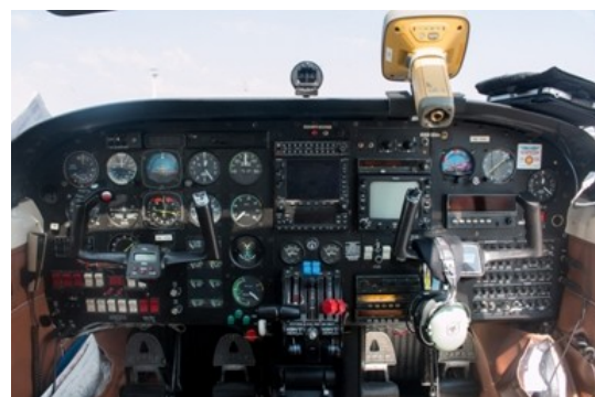
Figure 6. GNSS receiver mounted on the aircraft
