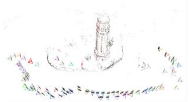
Figure 3: Sparse point cloud with camera positions
